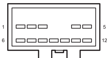
I2_FE Body W.H. Connector 2 Connecting Engine W.H.
