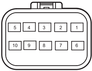
A9 Engine Control W.H. Connector Connecting Engine W.H.
